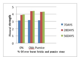
Figure 11: Comparison of flexural Strength of over burnt bricks and pumice concrete for the replacement 10% for 7, 28, 56 days
