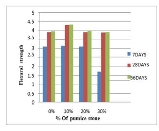
Figure 8: Variation of Flexural Strength gives the higher strength for the replacement 10% for 7, 28, 56 days by pumice stone
