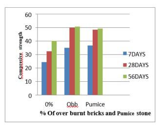
Figure 9: Comparison of compressive Strength of over burnt bricks and pumice concrete for the replacement 10% for 7, 28, 56 days
